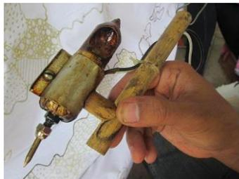
**Gambar 1.** Canting Elektronik
